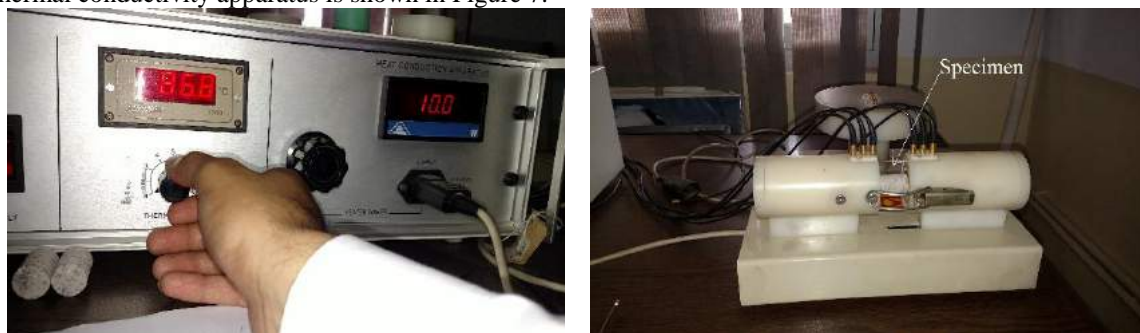
Figure 14 Electrical console of Helton Heat Conduction Apparatus (left), Linear Module Helton Heat Conduction Apparatus (right)
