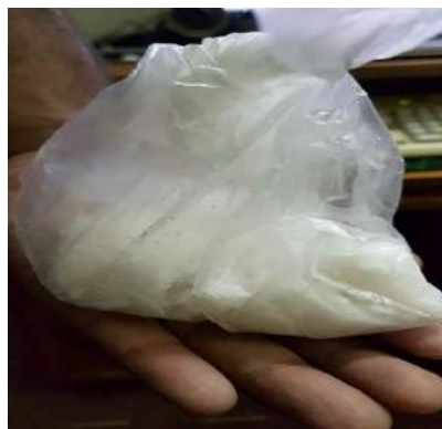
Fig 6: 0.5M per liter constituent of urea and calcium chloride (30.03 g urea, 55.49 g calcium chloride)
