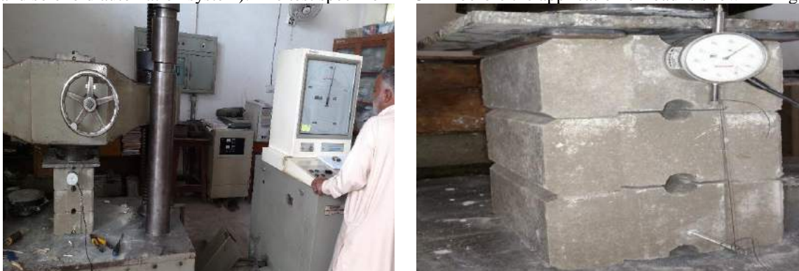
Figure 10 Deformation Dial Gauge and UTM connected with Data Acquisition System (left), Magnified picture of prism (right)
