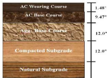
Fig. 5 Designed Cross-section of road.
