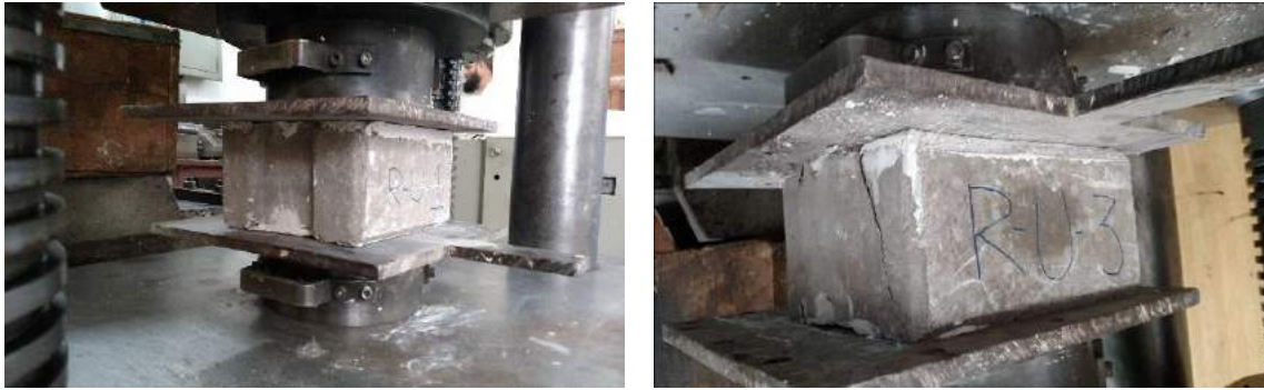
Figure 9 Hydraform Block Capped with Gypsum (left), Hydraform Block after Uni-axial Compression Failure (right)
