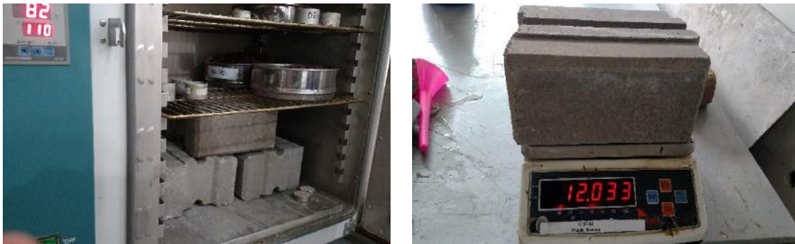
Figure 13 Hydraform blocks in Electric Oven (left), Hydraform block on Electric Balance after fully saturated in water (right)
