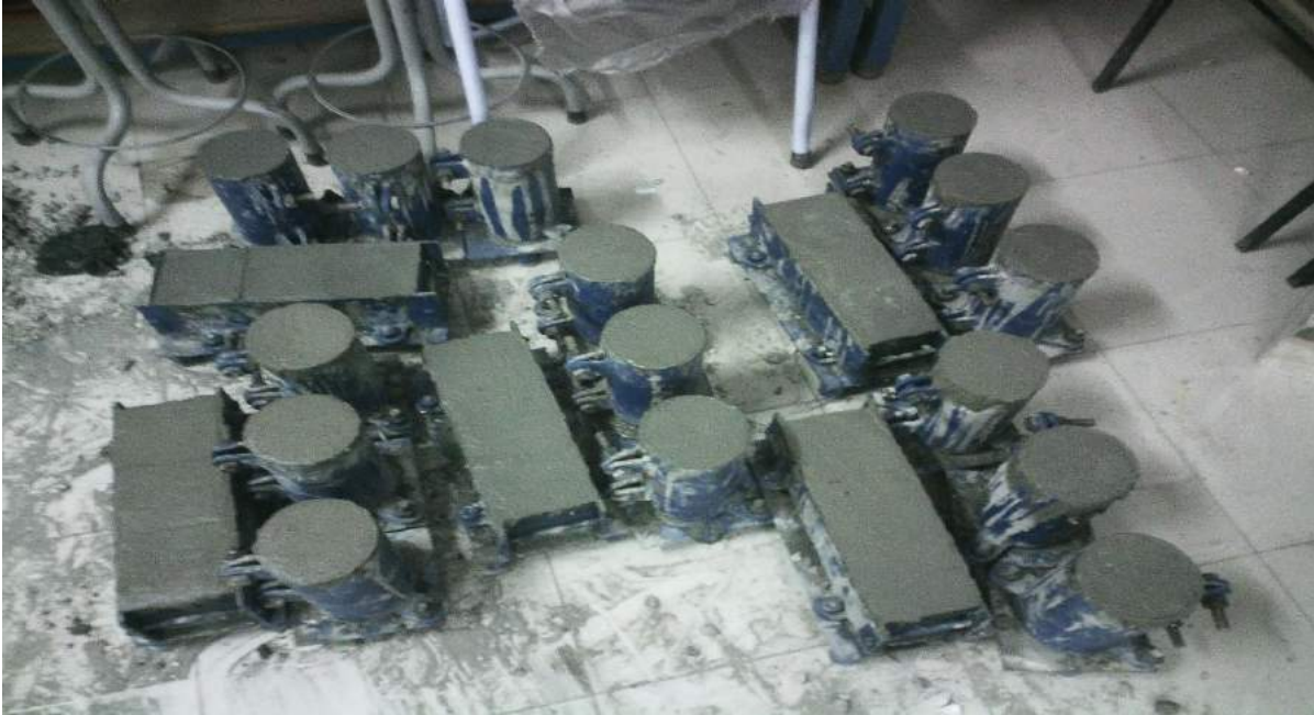
Figure 1. Casting of concrete cylinders and cubes
