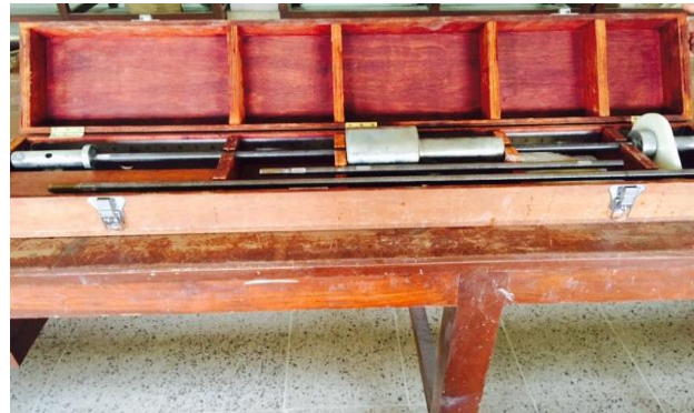
Fig. 7: Dynamic Cone Penetrometer Test (DCPT)
